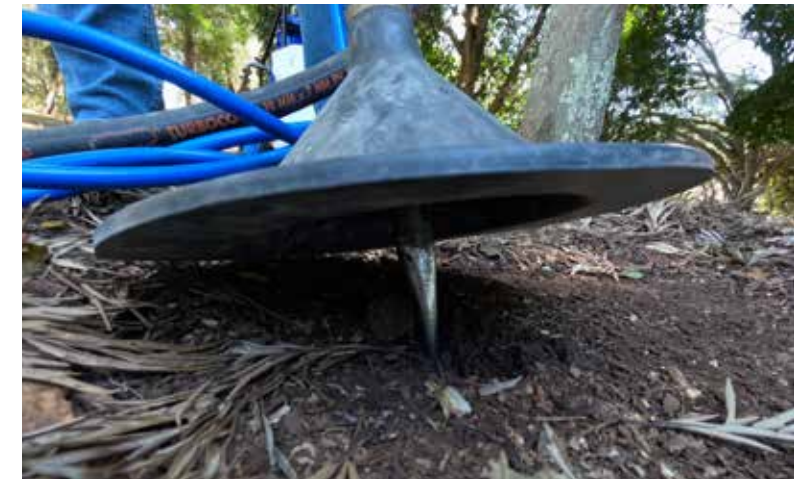
Air Spade needle that is injected into the ground and is used to disperse the air and other material into the soil.
