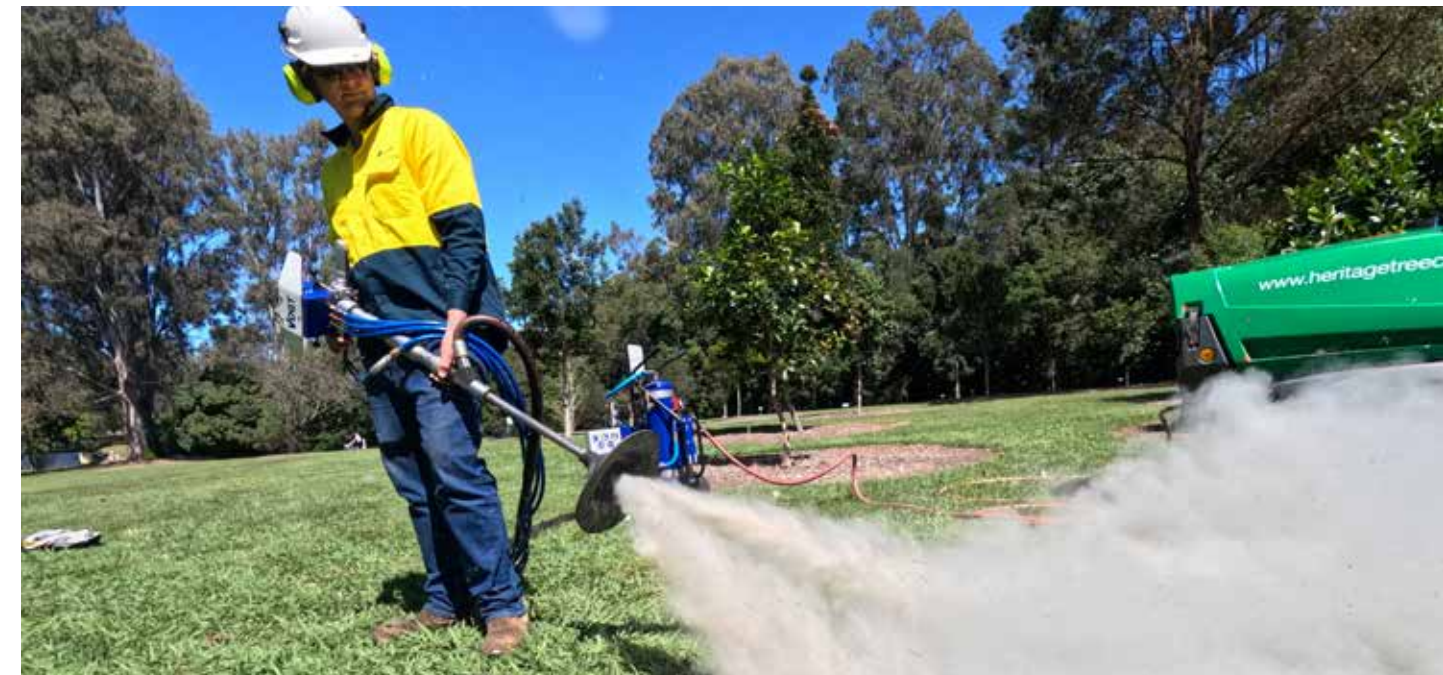
Air Spade operator demonstrating the process of decompaction that would normally occur underground.
