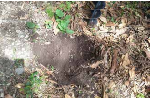
Preparations for the retrieval of soil samples along with a visual inspection of the soil layers.
