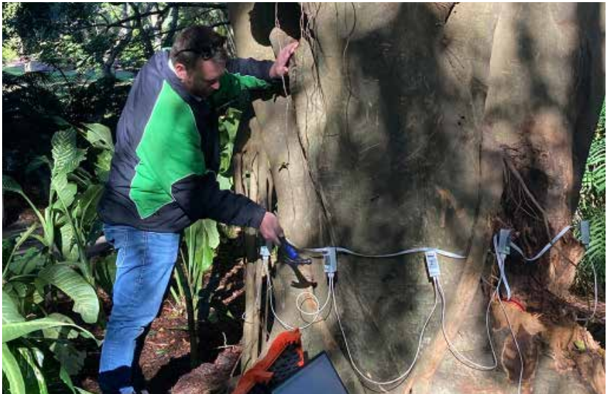
An arborist fixes the tomograph nodes in place, preparing to make an assessment on whether the tree has any cavities of structural weakness' inside.
