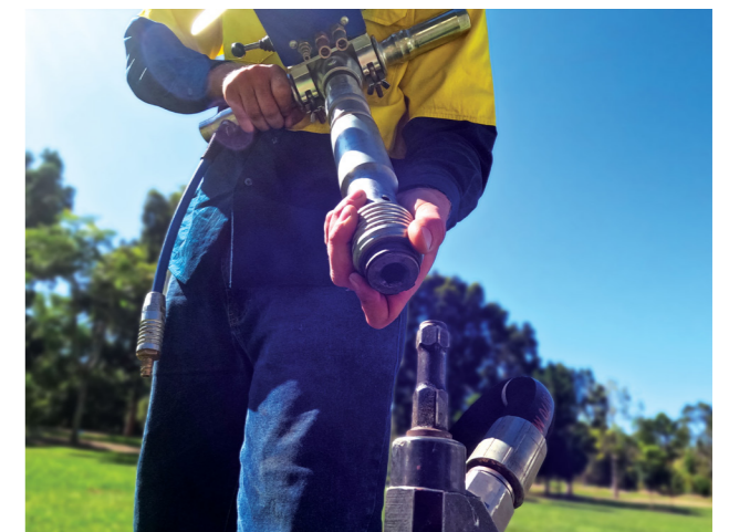
A VOGT needle that is injected into the ground and is used to disperse the air and other material into the soil.
